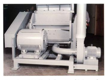
Heavy duty motor and long lasting, wear resistant evacuation blower can be integrally mounted at the base of the machine,
