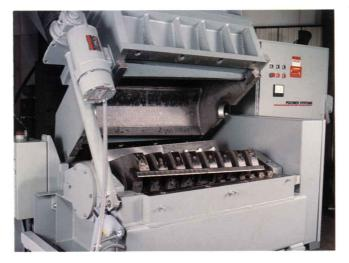
Split chamber design with power assisted tilting hopper provides easy access for knife adjustment and cleanout. Cutting chamber and screen cradle are interlocked for safety.
