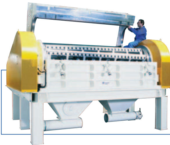
ALPINE ROTOPLEX® GRANULATOR 90/300 Ro ROTOR WIDTH 3000 mm ROTOR DIAMETER 900 mm
