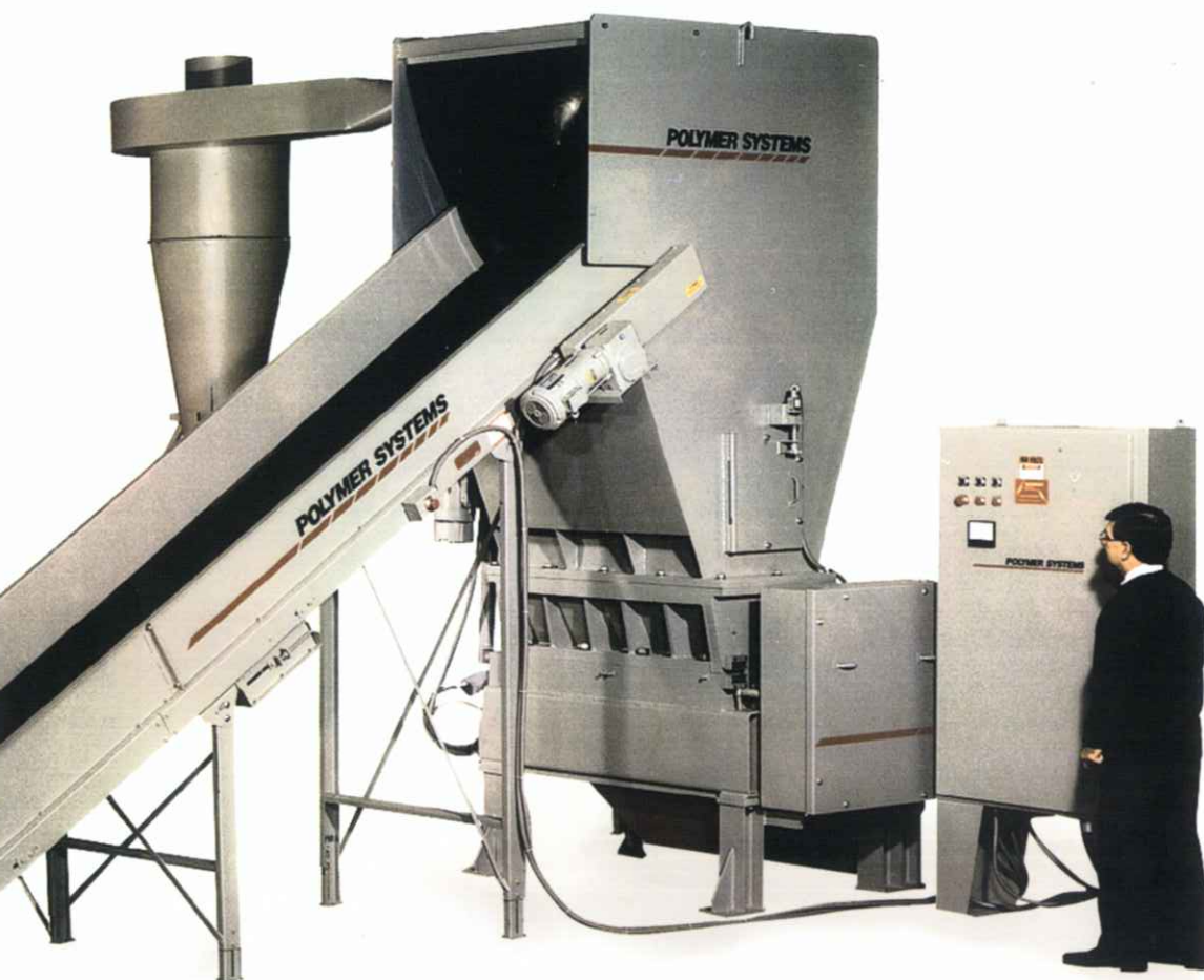
Heavy Duty Model 2441 supplied as a complete material recovery system for a high volume application.
