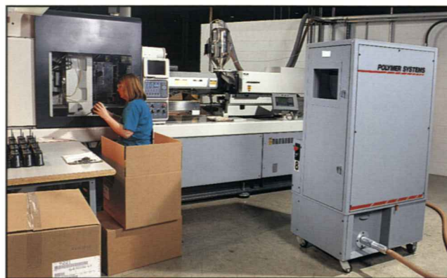
Vacuum bin under granulator evacuates regrind for blending with virgin resin in automated recovery system.
