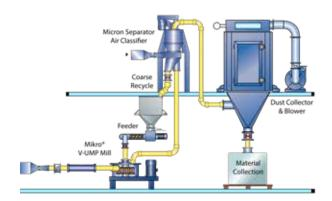
Hosokawa's V-UMP Mill systems can incorporate high-efficiency air classifiers for applications where ultra-fine grinding is required, providing extremely tight particle size distributions and the ability to make a fine and coarse end product.
