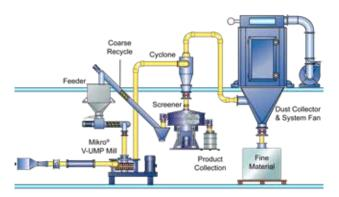
Hosokawa can install a cyclone and a screener inline with your V-UMP Mill for material separation and collection, preventing oversize particles and ensuring powder tcp size.
